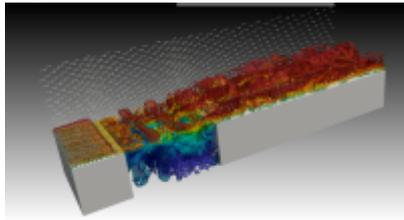
8. 3D shear-layer driven cavity flow with a constant forcing source
