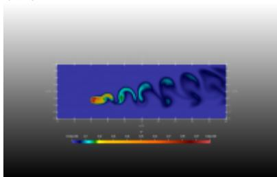
11. 2D flow around a heated square-cylinder -  $Re_h = 50$ ,  $Ra = 5.10^6$
