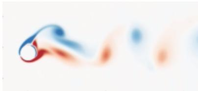
10. 2D flow around an oscillating cylinder -  $Re_D = 185$
