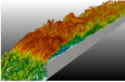
4. **3D forward-facing step flow -  $Re_h = 8000$  (turbulent inflow)**
