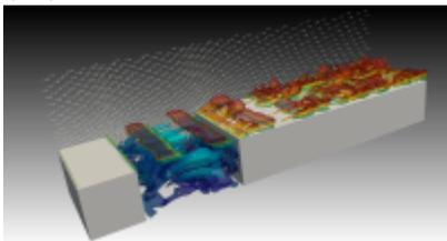
7. **3D shear-layer driven cavity flow -  $Re_{L_c} = 7826$**
